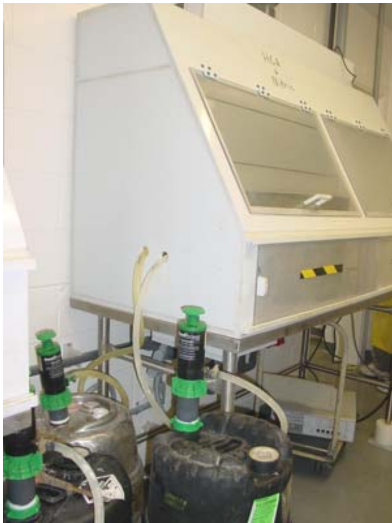
After: GoatThroat delivers technical grade HCl and Nitric Acid, plumbed in through side of fume hood, dispensed with remote tap. Acid cost reduced to $.20 per unit.
