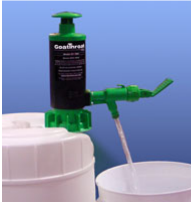
Figure 1: With the new transfer method, it was now possible to meet North Carolina's closed-used safety codes for dispensing liquids from five-gallon containers on the fourth floor.
