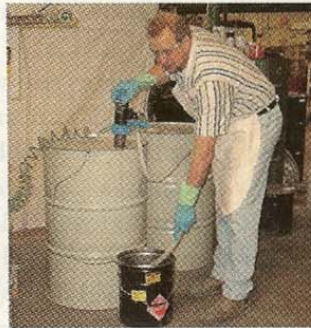
Pressure-action drum pumps facilitate fluid transfers.
