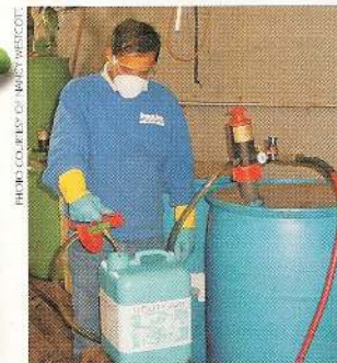
Pressure-action drum pumps facilitate fluid transfer.
