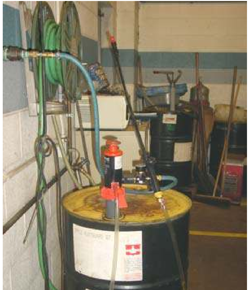
Applying rust-inhibitor with a sprayer using GoatThroat Pump and BillyGoat Shop Air Adapter
