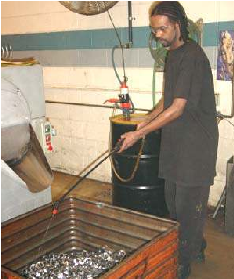
Applying rust-inhibitor with a sprayer using GoatThroat Pump and BillyGoat Shop Air Adapter
