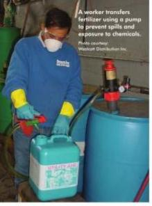
the precise control of product the pumps allow enables exact filling of measuring containers to the desired fill lines for more consistent results in mix tanks.
