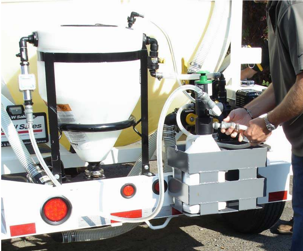
Photo Four: Mixing/loading system with GTP suction/extraction unit in place
