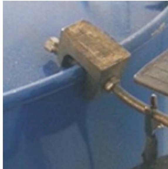
Close up of the barrel side Held in place by a clamp with a thumb screw
