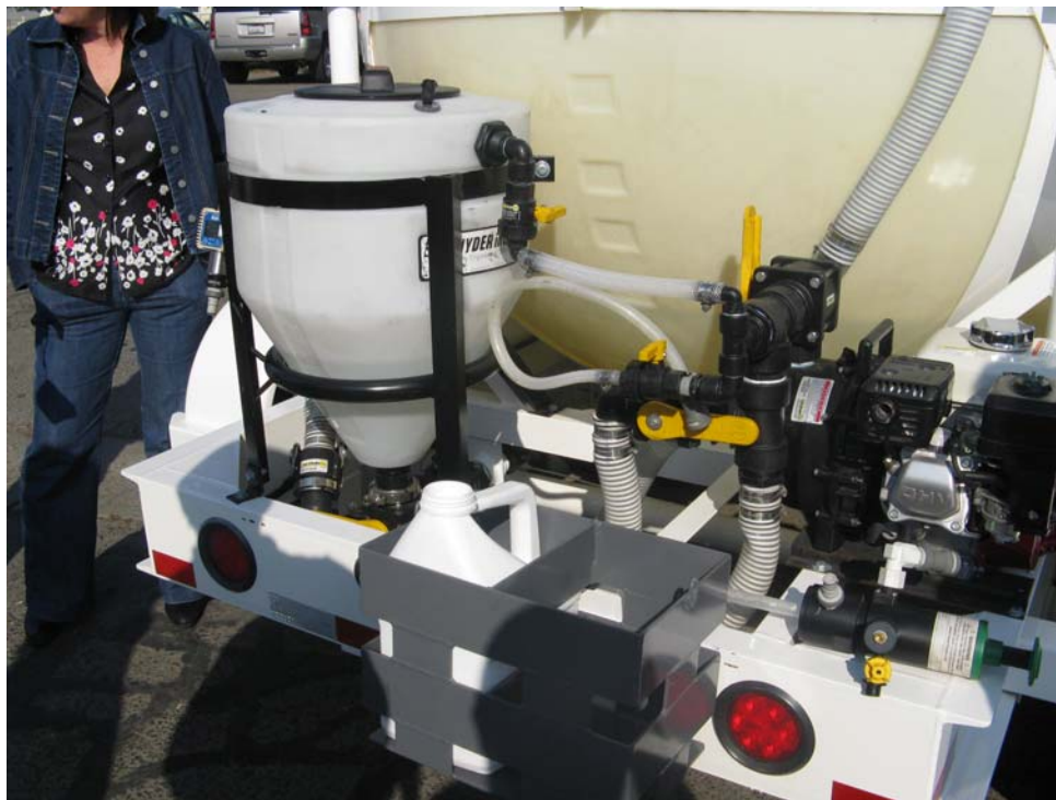
Photo Three: Mixing/loading system without GTP suction/extraction unit
