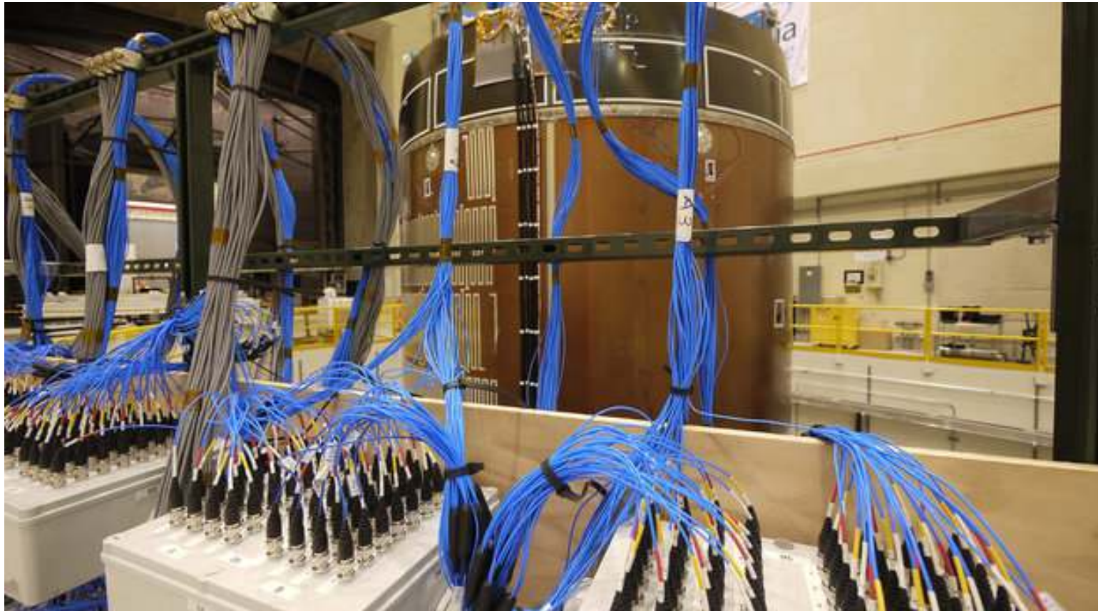
Figure 6: Sensing Orion—European Service Module test article.
