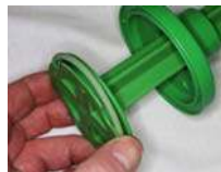
Fitting the O-ring to the Piston
