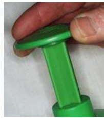
Fitting the Piston Screw Top to the Piston
