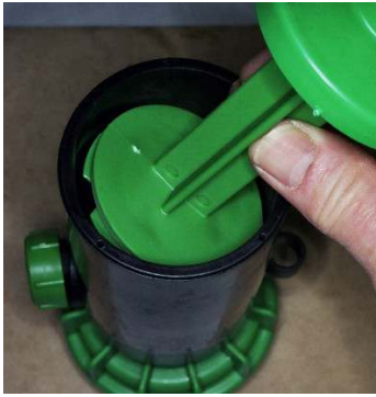
Fitting the Piston into the Pump Body
