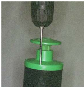
Fitting the Body Cap Screws
