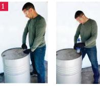
Stand with feet shoulder width apart approx. 6-8" away from pump to install stand-off and pump.
