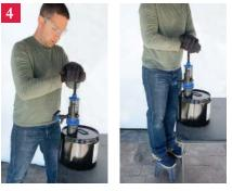
When operating with a 5-gal drum: Set drum on a stable surface at least 27.5" in height. Then follow steps 1-3.
