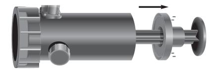
2 Use flat head screwdriver to pry O-ring from piston. Lubricate inside body barrel with small amount of Molykote111 compound. and fit replacement o-ring it to piston, making sure it is seated properly in the groove.
