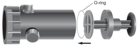
**3** Replace piston. Align tab on underside of cap with hole on pump body noting line-up dowl, then replace and tighten screws.
