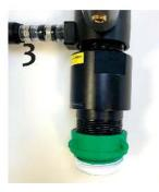
If used, thread pump adapter into butress adapter for a tight fit. Keep this assembly together always.
