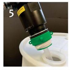
Remove closure from the thick thread side of the barrel. Install pump and tube assembly at a slight angle into the barrel.
