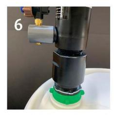
Straighten up pump assembly, and thread onto barrel making an air-tight fit. TO REMOVE PUMP: turn green buttress adapter only.
