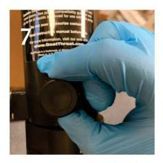
Ensure pressure release knob is tightly closed for operating.
