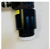
Wrap pump adapter with several layers of teflon tape.
