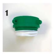
If used, wrap buttress adapterwith several layers of teflon tape.
