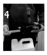
Push siphon tube into bottom of pump, teflon toward the pump. Turn it during installation for the best fit.
