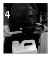
If used, wrap buttress adapterwith several layers of teflon tape.
