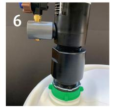
Straighten up pump assembly, and thread onto barrel making an air-tight fit. TO REMOVE PUMP: turn green buttress adapter only.
