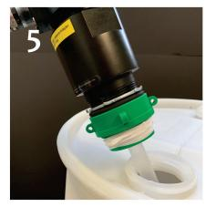
Remove closure from the thick thread side of the barrel. Install pump and tube assembly at a slight angle into the barrel.
